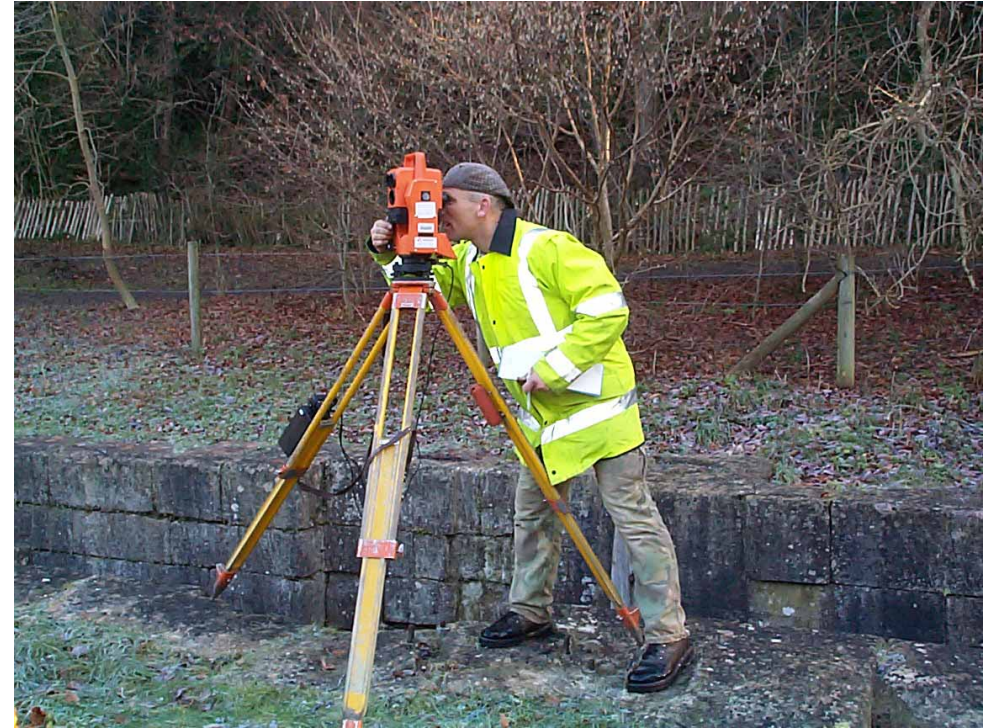
RICHARD HIGNETT WITH THE 'TOTAL STATION' AT LOCK 15
