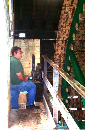
THE SLUICE GEAR WHICH CONTROLS THE WATER FLOW TO THE WHEEL
