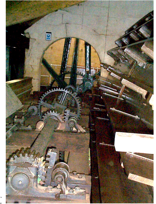
THE SLUICE GEAR WHICH CONTROLS THE WATER FLOW TO THE WHEEL
