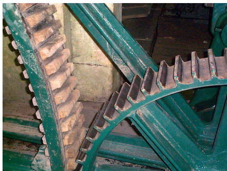
OAK TEETH ON THE PIT WHEEL (left) MESHING SMOOTHLY WITH THE IRON TEETH OF THE CRANKSHAFT GEAR (right)
