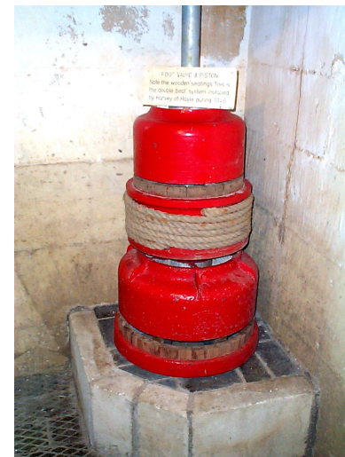
A PISTON WITH VALVE (Left) AND THE FOOT VALVE INSPECTION COVERS (Right)
