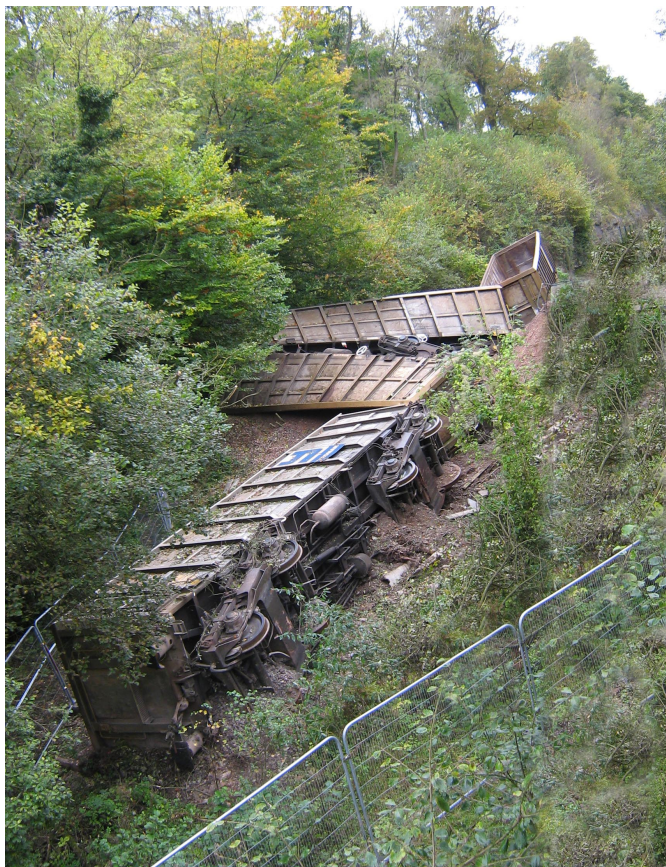
Left: DERAILED STONE WAGGONS TUMBLED DOWN THE RAILWAY EMBANKMENT
