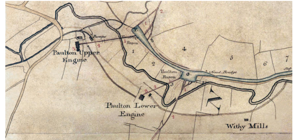
THE AREA AROUND THE TERMINUS OF THE MAIN LINE OF THE CANAL From the Canal Company Map, showing the leat from the Cam Brook passing through the Engine Pits towards Withy Mills. Paulton Foundry, completed in 1807, was probably already under construction in the space marked by the word "Lower"
