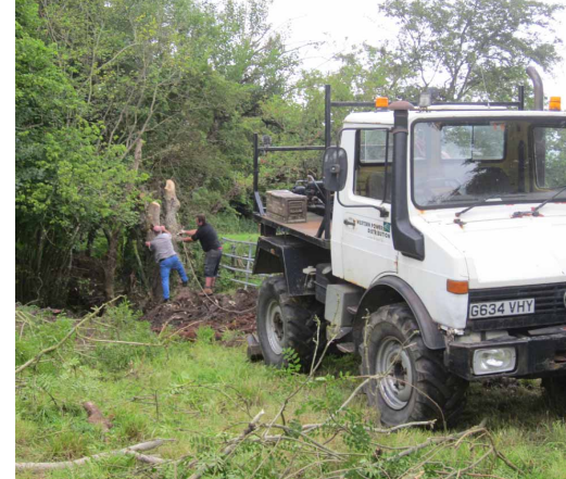
A 'UNIMOG' EQUIPPED WITH A POWERED WINCH AND A BULLDOZER BLADE (TO PREVENT SLIPPING) TOWING OUT A DEAD TREE STUMP
